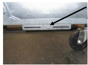
**Figure 1**: Attach alignment bracket to bottom of ATO box brace.
